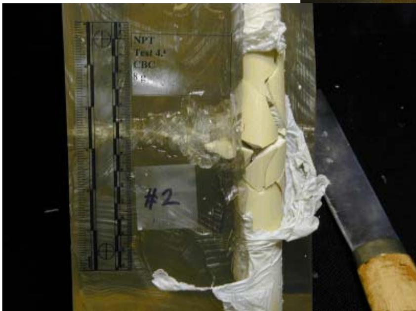
**Figure 12 Synthetic generic bone tube imbedded in 10% gelatine and penetrated by a 9 mm FMJ bullet. The silicone “periosteum” has been removed to more clearly show the fracture. Note the lack of longitudinal fractures in the bone tube.**
