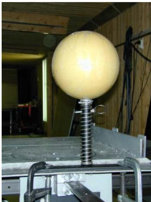
**Figure 13 : Police technical centre artificial flexible atlas vertebra for mounting a skull for helmet testing.**
