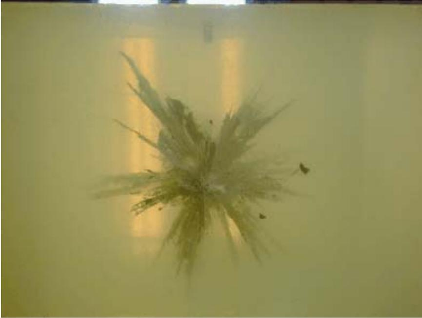
**Figure 10: An example of the wound channel of an expanding 5.56 mm bullet in 10% gelatine as seen from the direction of the gun. A fragment has penetrated transversally about 50 mm from the bullet path.**
